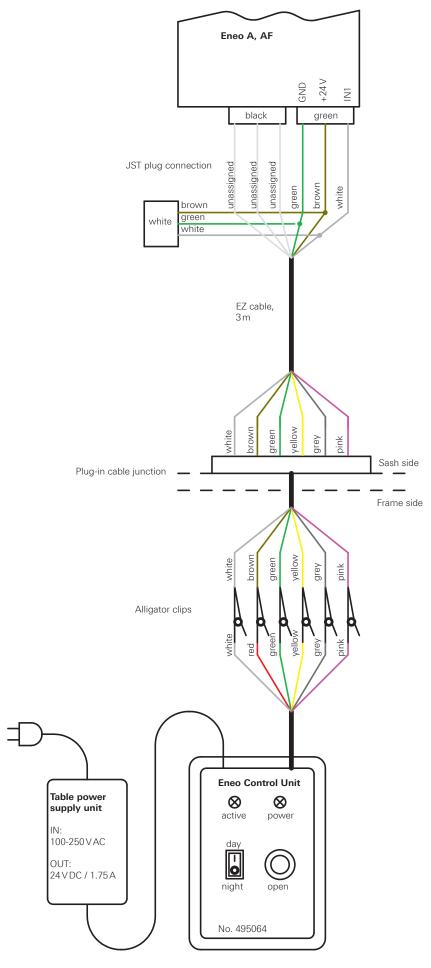
**Connector / cable assignment** white: IN1 / input 1 (OPEN)
