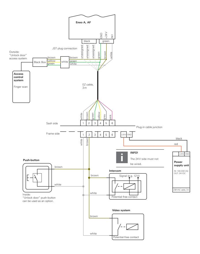
Finger scan cable assignment (between JST connector and Black Box) brown: +24V
