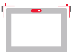
Tilt-Only hardware Without restrictor and cleaning stay Tilt stay(s) at the top
